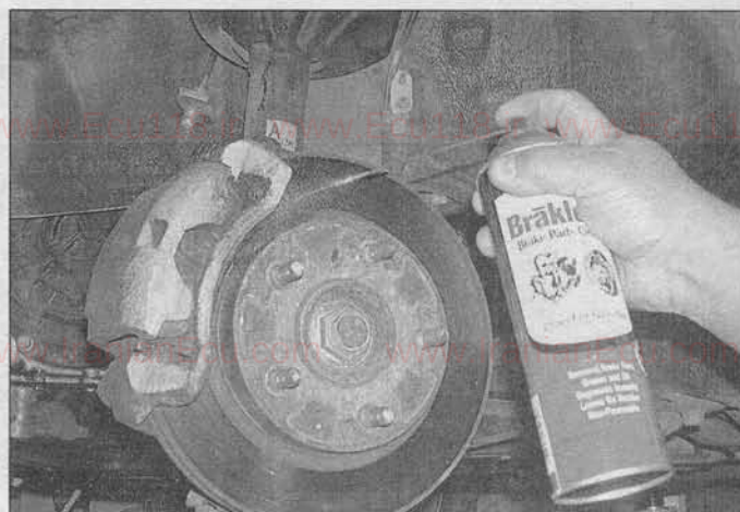
3.6a Before removing anything, spray the disc, caliper and brake pads with brake system cleaner to remove the dust produced by brake pad wear - DO NOT blow the dust off with compressed air!
