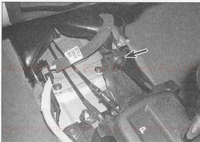
4.7 To remove the shift cable, remove the large C-clip retainer (arrow) from the shift bracket
