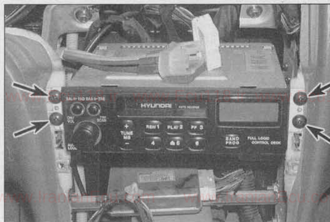
11.3a Remove the screws (arrows) to remove the radio
