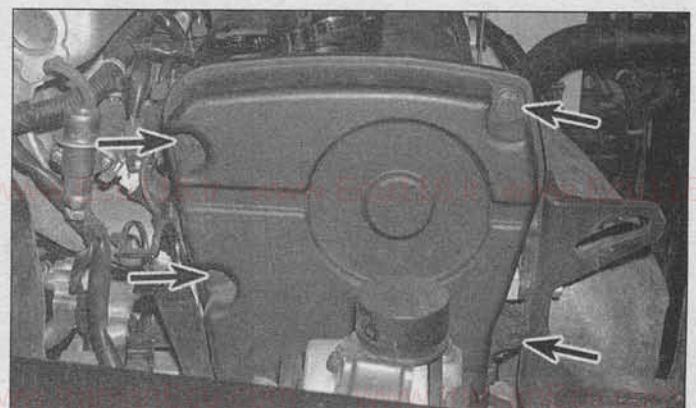
4.5 Remove the bolts (upper arrows) that attach the upper timing belt cover to the valve cover; to remove the upper timing belt cover, remove the two lower bolts (lower arrows) as well
