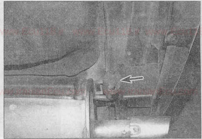
27.2b Check each exhaust system hanger (arrow) for damage and cracks
