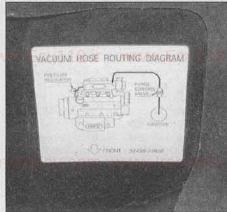
1.7b Vacuum hose routing diagram of the emissions system vacuum hoses
