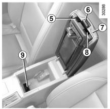
Centre console storage compartment with two layers (depending on the vehicle)
