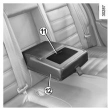
Cup holder 11 Lower the central rear armrest and press 11 to allow the cup holder to be used.
