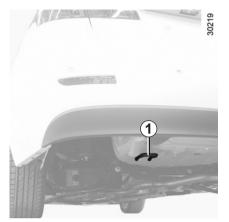
Only use rear towing point **1** and front towing point 4 (never use the drive shafts). These towing points may only be used for towing: never use them for lifting the vehicle directly or indirectly.
