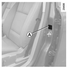
The tyre pressure is indicated on label **A** affixed to the vehicle's body. Open the door to read it.
