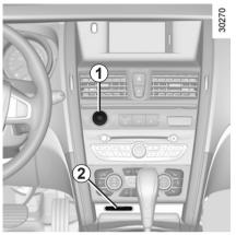
**Remote control RENAULT card** When you get into the vehicle, insert the RENAULT card fully into card reader 2. To start, press button **1**. If a gear is engaged, depress the clutch pedal to start the vehicle.
