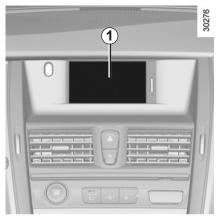
With the ignition on, the time and, depending on the vehicle, the exterior temperature are displayed on display 1.
