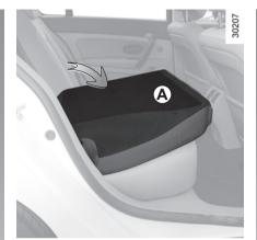
To put the seatback back in position, raise it then check that it is locked correctly.
