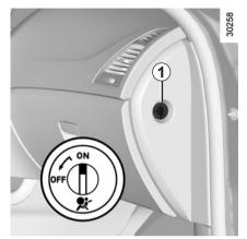
**Deactivating the front** passenger air bag (on equipped vehicles)
